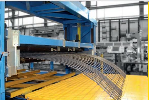
Curved bespoke mesh for precast tunnel and wind turbine elements
