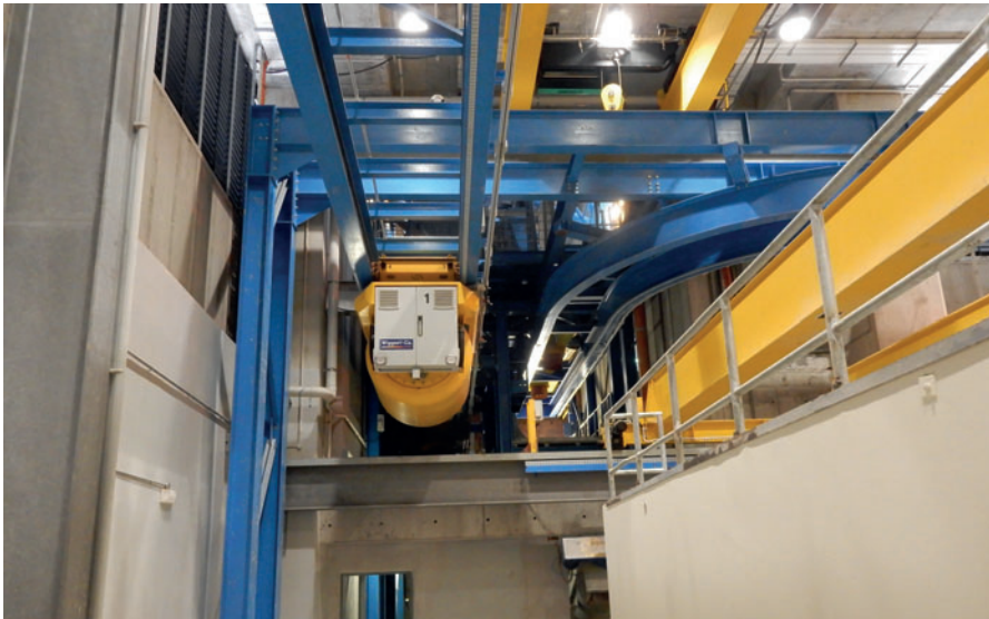
Even the fresh concrete is delivered automatically to the production lines by means of various bucket conveyors.
