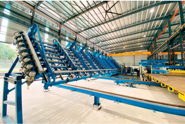
The M-System Evolution is an advanced mesh welding plant that produces customized reinforcement mesh for precast elements.
