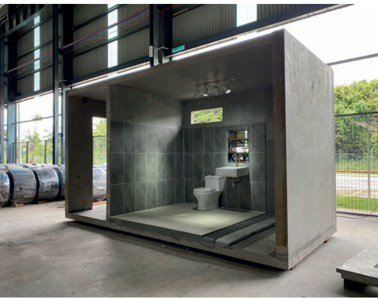
IJM IBS PPVC: Prefabricated and fully equipped with architectural finishes, ready for efficient delivery to the construction site.
